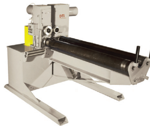
Power Driven Uncoiler For Large Diameter Applications
