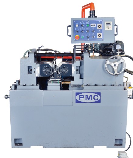
▲ PM-60VS with Precision Center Rest Fixture for Spline Rolling
