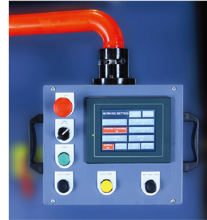
Centralized Control Panel incorporates with PLC & HMI
