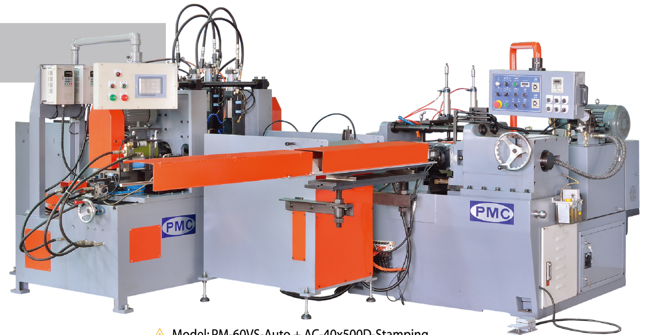
▲ Model: PM-60VS-Auto + AC-40x500D-Stamping (Fully-Automatic Double-Ends Chamfering + Stamping + Thread Rolling Production)
